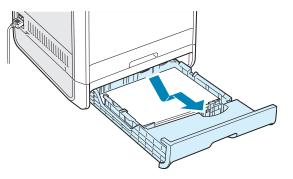
8 If you see the jammed paper, remove the paper from the printer by gently pulling it straight out.
